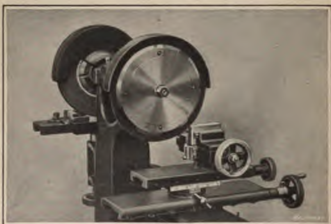
Fig. 7. Geometric Chaser Grinder set up for Grinding Throat of Hobbed or Tap-formed Chaser
